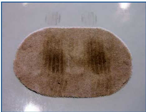
Carpet pad placed to prevent tire staining.
