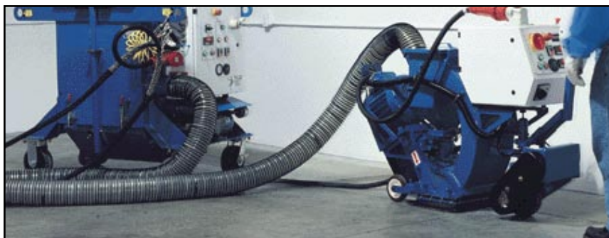
General floor preparation/cutting and cleaning control joints / portable vacuum blasting.
