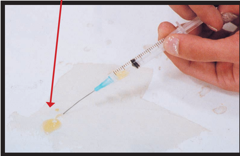
The moisture bubble problem was so severe, we were able to pull almost 2ml out of one bubble. Again, fortunately, this was isolated to one small area of the hangar.
