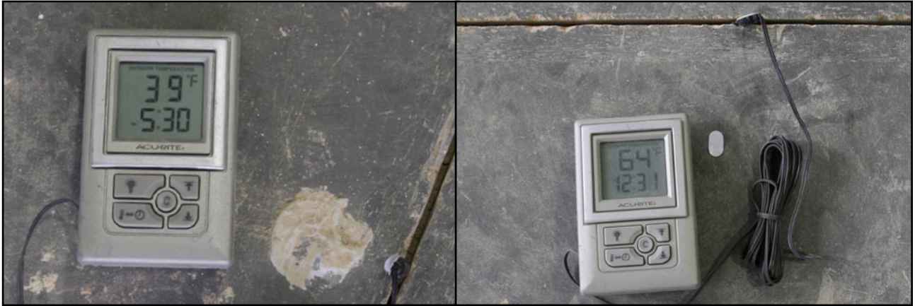
The concrete slab temperature varied from 39° F near the front doors to 64° F underneath the heaters.
